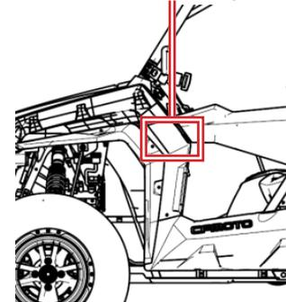
Each trouble code consists of 2 digits, denoted by the times of long flash and short flash of EPS MIL indicator. If there is a failure, the EPS indicator will start to flash. Do NOT switch off the machine. Check the flash sequence of EPS indicator. Write down the flash sequence and contact your dealer for diagnosis. Your dealer has the special tool required to diagnose, repair and clear trouble codes. Any codes will disappear once the problem has been diagnosed and repaired by your dealer.
